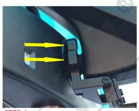
STEP 4 - Position the mount towards the front of the vehicle as far as it will go. Rotate the mount so it is parallel with the bottom of the mirror. Tighten the clamp screw untill the mount is securely attached to the mirror stem. Do not over tighten the clamp screw.
